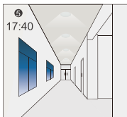
The light automatically turns on at 25% when natural light is insufficient (no motion).
