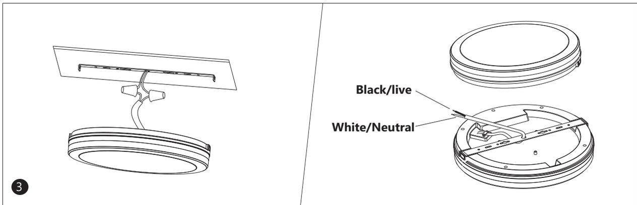
3. Connect black wire to live wire, white wire to neutral wire, and secure using wire nuts.
